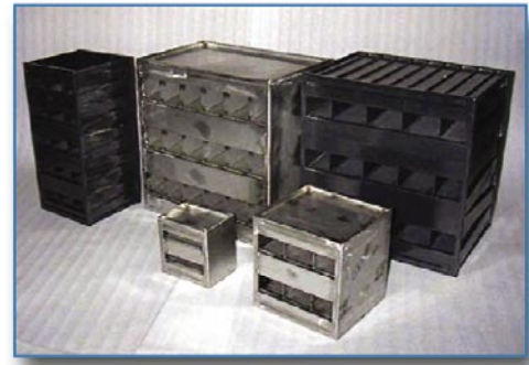
Figure 5-9 Charcoal filter beds
